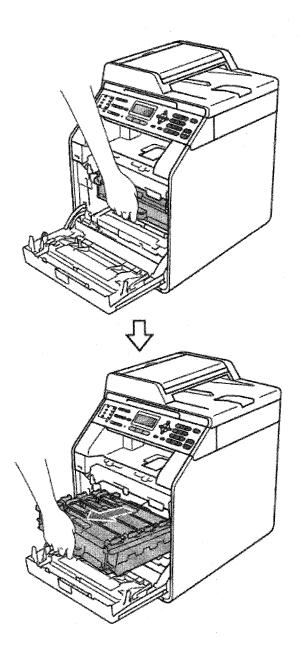
Hold the handle of the toner cartridge and slightly push it toward the machine to unlock it. Then pull it out of the drum unit. Repeat this for all the toner cartridges.
