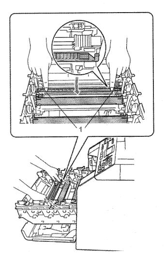
Clean the corona wire inside the drum unit by gently sliding the green tab from left to right and right to left several times.
